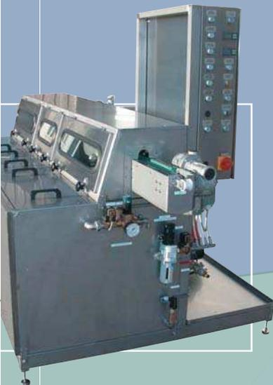
**VL** cleaning machine with vertical gate
