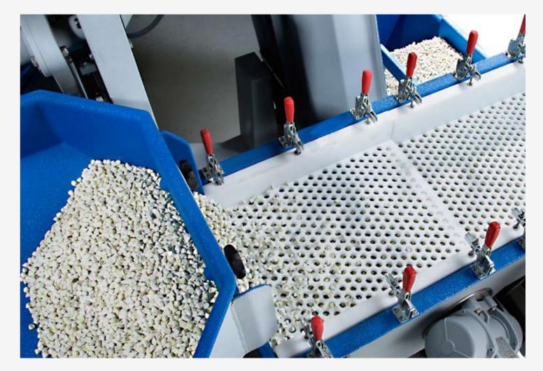
Separation of workpieces and abrasives
