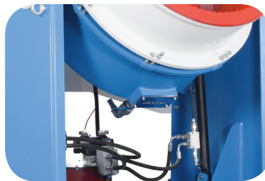
AutoTilt System with hydraulics Hidrolik Sistem Otomatik Devirme
